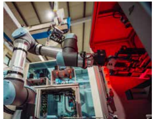
ZDZW is developing a system for inspecting parts produced by plastic injection moulding processes, demonstrated at the GLN facilities
