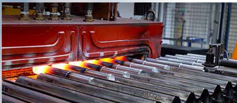
The project is improving the manufacturing process of high-quality large metric fasteners, using induction heat treatment, for the wind and aerospace industry, demonstrated at the ERREKA facilities
