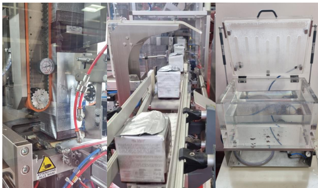
FIGURE 16: VERTICAL BAGS FORMING AND THERMO-WELDING. WATER IMMERSION TEST UNIT FOR SEALING CONTROL.
