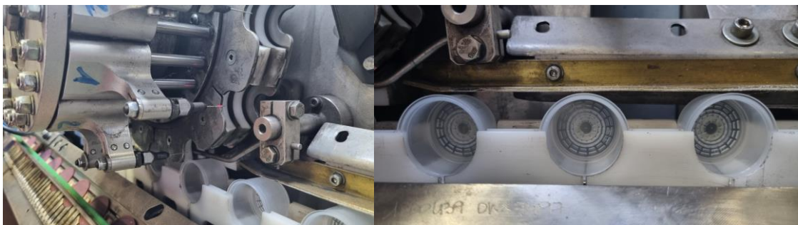
FIGURE 14: DRUM WITH NEEDLES FOR PERFORATING THE CAPSULE BODIES AND PERFORATED BODIES ON THE OUTPUT LINE
