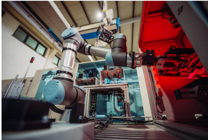
FIGURE 8: Installed Automatic Inspection for Plastic Injected Products
