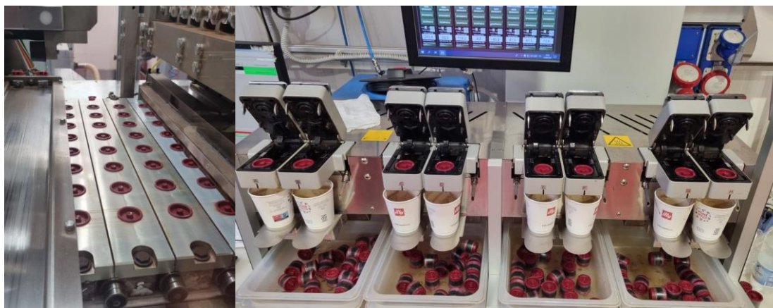
FIGURE 15: Capsules Exiting from Lid Sealing. Multi-head Coffee Machine for Destructive Testing of Capsule Sealing
