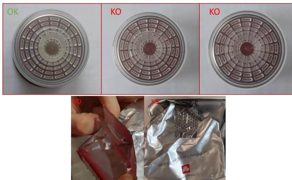
FIGURE 13: FAULTY COFFEE CAPSULES AND DEFECTED CAPSULE BAGS
