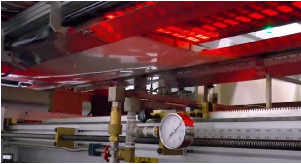
FIGURE 17. A VIEW OF THE HEATING ELEMENT ARRAY AND THE PLASTIC SHEETS
